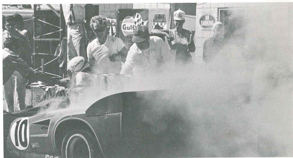
Parsons exits his burning Lola in the pits. The Lola-Chevy intake manifold had cracked and everything had so overheated the fiberglass rear body section caught fire.
